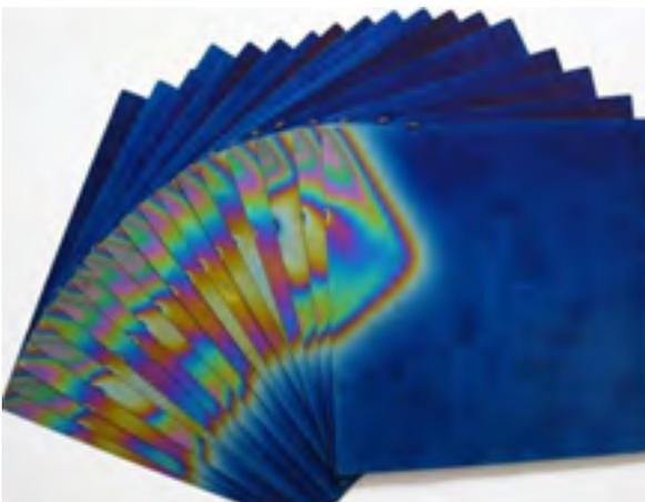
Figure 1: Out-of-spec colors due to SiNx process deviation – color variation due to different SiNx layer thicknesses.
